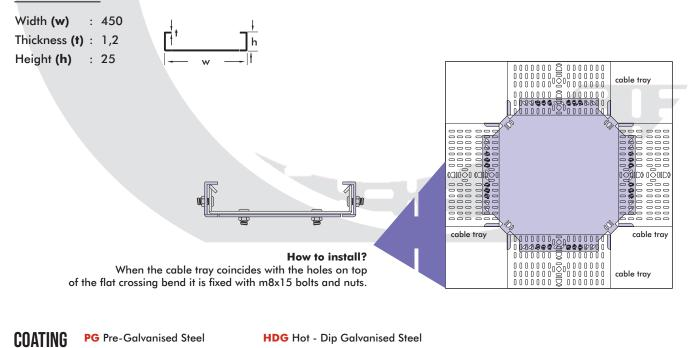
**EPC** Electrostatic Powder Coating **SS** Stainless Steel
