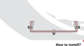
When the cable tray coincides with the holes on top of the flat crossing bend it is fixed with m8x15 bolts and nuts.
